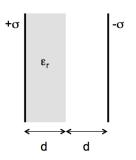
We insert a slab of linear dielectric material of dielectric constant  $\epsilon_r$  and thickness d next to the positive plate in a parallel plate capacitor. The distance between the plates is 2d, their area is A and they carry a (free) charge density  $\pm \sigma$ .
