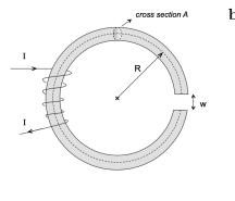
b) To increase the energy that can be stored in the inductor, we have to find a way of increasing the saturation current while keeping L constant. This can be done by introducing an air gap of width w into the core. We take  $w \ll R$ , so that we can neglect magnetic fringing, that is to say the bulging out of the magnetic field lines as they enter air from the magnetic material.
