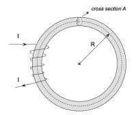
We consider a toroidal core made of an iron alloy with cross sectional area A and radius  $R \gg A^{1/2}$ . We make an inductor from the core by wrapping around it N turns of a wire carrying a current I, to use it as an energy storage device.
