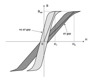
c) Some of the energy stored in the inductor can be recovered by decreasing the current back to 0. The figure shows the B - H curves (hysteresis loops) measured on a toroidal core without and with gap (the straight lines inside the loops are the magnetization curves).
