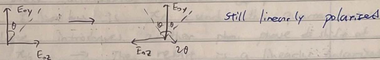
but the ~~direction of p~~ plane of polarisation is rotated by  $2\theta$ , where  $\theta$  is the angle between the plane of polarisation and the ~~slow~~ component. Vertical ✓
