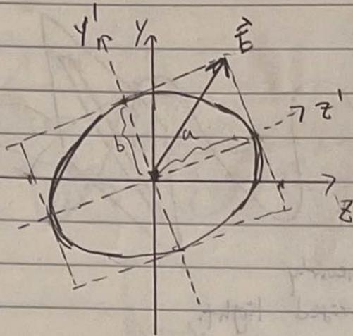
Orient the quarter-wave plate such that the axis of the plates matches the ~~axis~~ of major and minor axes of the ellipse.  $y', z'$  ✓
