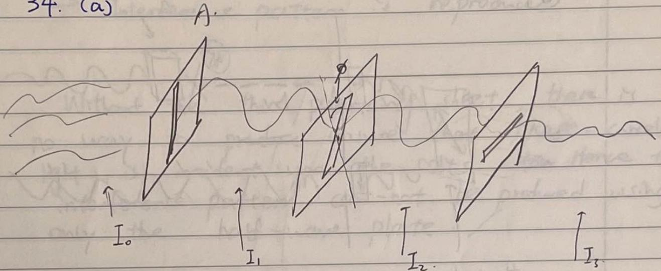
$$I_1 = \frac{1}{2} I_0, \quad I_2 = I_1 \cos^2 \phi, \quad I_3 = I_2 \cos^2 \left( \frac{\pi}{2} - \phi \right) = I_2 \sin^2 \phi$$
