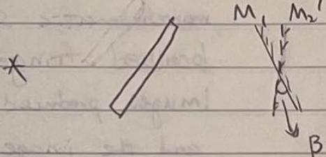
In this configuration  $M_1$  and  $M_2$  act like a wedge and ~~produces~~ produce equally spaced fringes.  $M_1$  and  $M_2$  needs to have very small separation and needs to be slightly ~~tilted~~ tilted with respect to each other.
