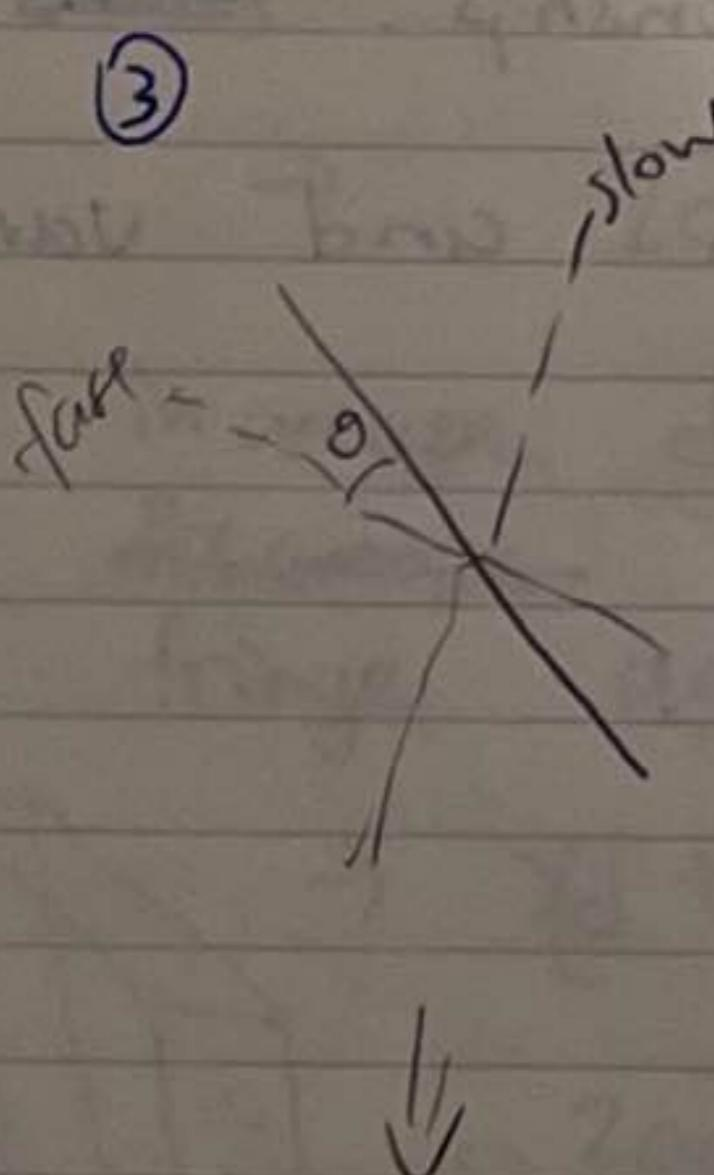
Now orient the second  $\lambda/4$  plate such that its fast axis makes an angle  $\alpha$  w.r.t the polarisation direction (Angle  $2\alpha$  w.r.t the first  $\lambda/4$  plate)
