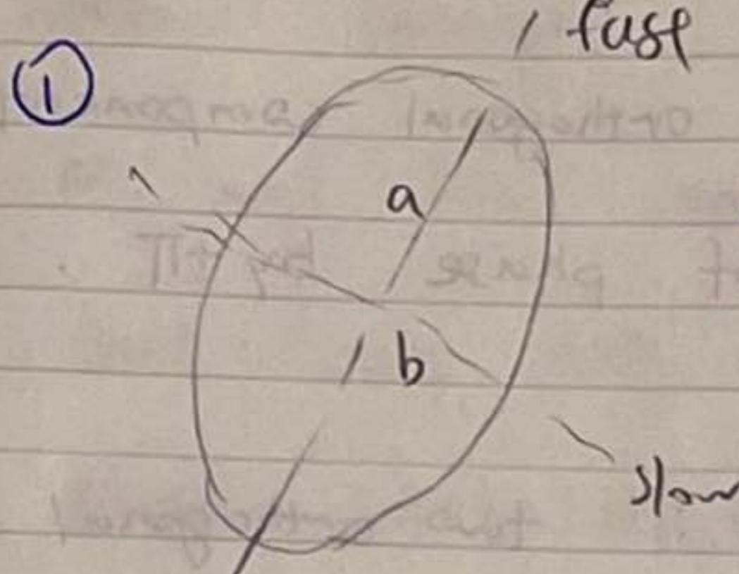
Orient the fast and slow axes such that they coincide with the major and minor axis of the elliptically polarised light
