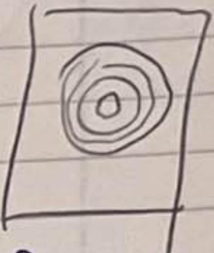
The Fabry-Pérot etalon consists of two parallel plates that can both reflect and transmit light. The two plates turn the incident beam into multiple beams with certain phase difference and ~~they~~ interfere to give circular fringes.
