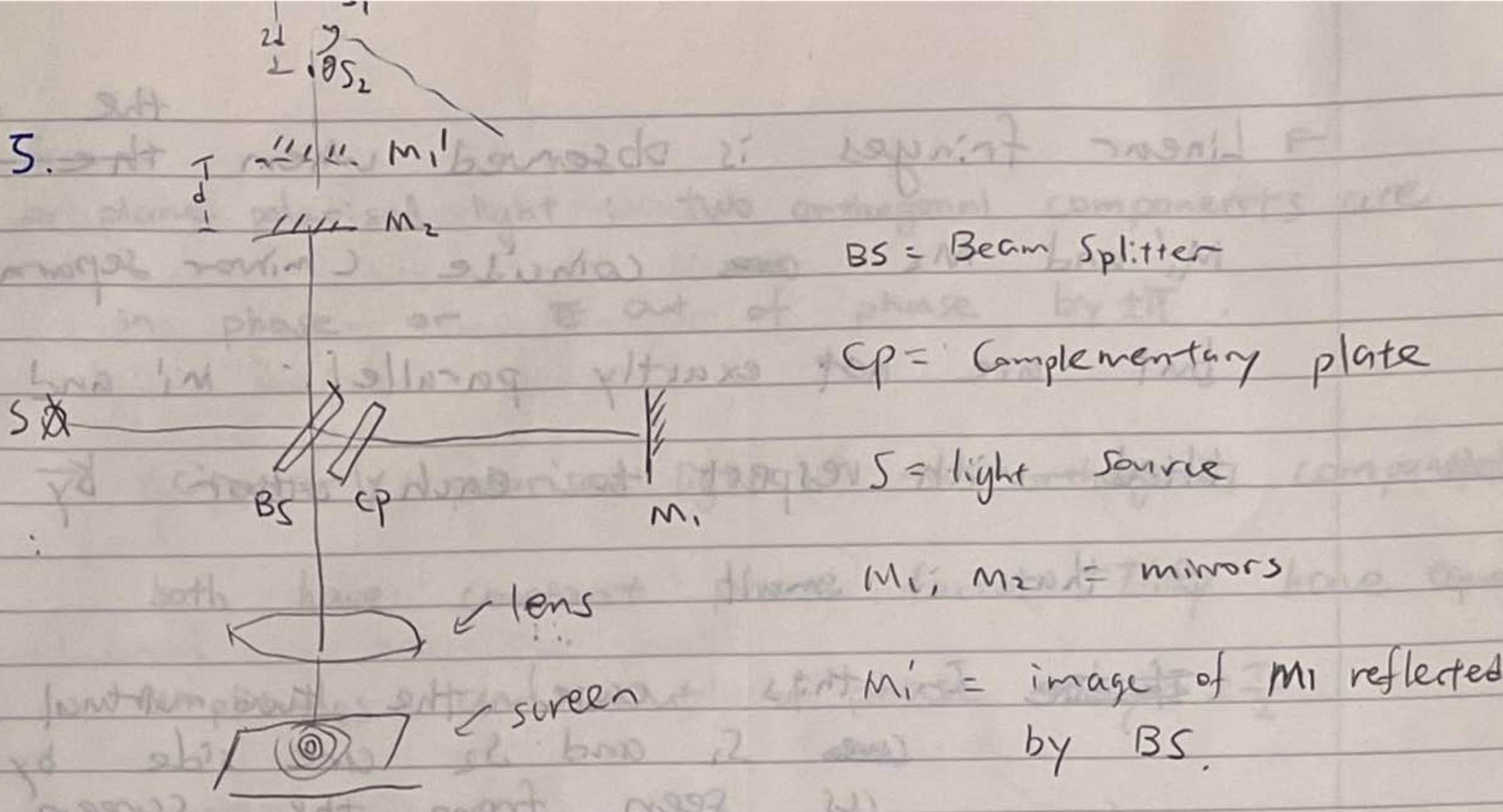
→ Circular fringes are formed when  $M_1'$  and  $M_2$  are exactly parallel and have a separation
