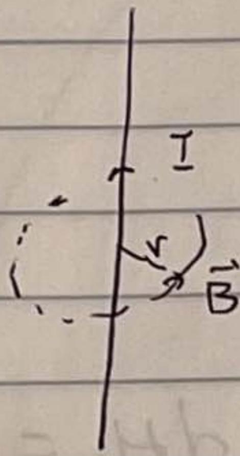
$$\begin{aligned} \vec{B} &= \frac{\mu_0 I}{2\pi r} \hat{\theta} = \vec{\nabla} \times \vec{A} \\ &= \left( \frac{\partial A_r}{\partial z} - \frac{\partial A_z}{\partial r} \right) \hat{\theta} \end{aligned}$$
