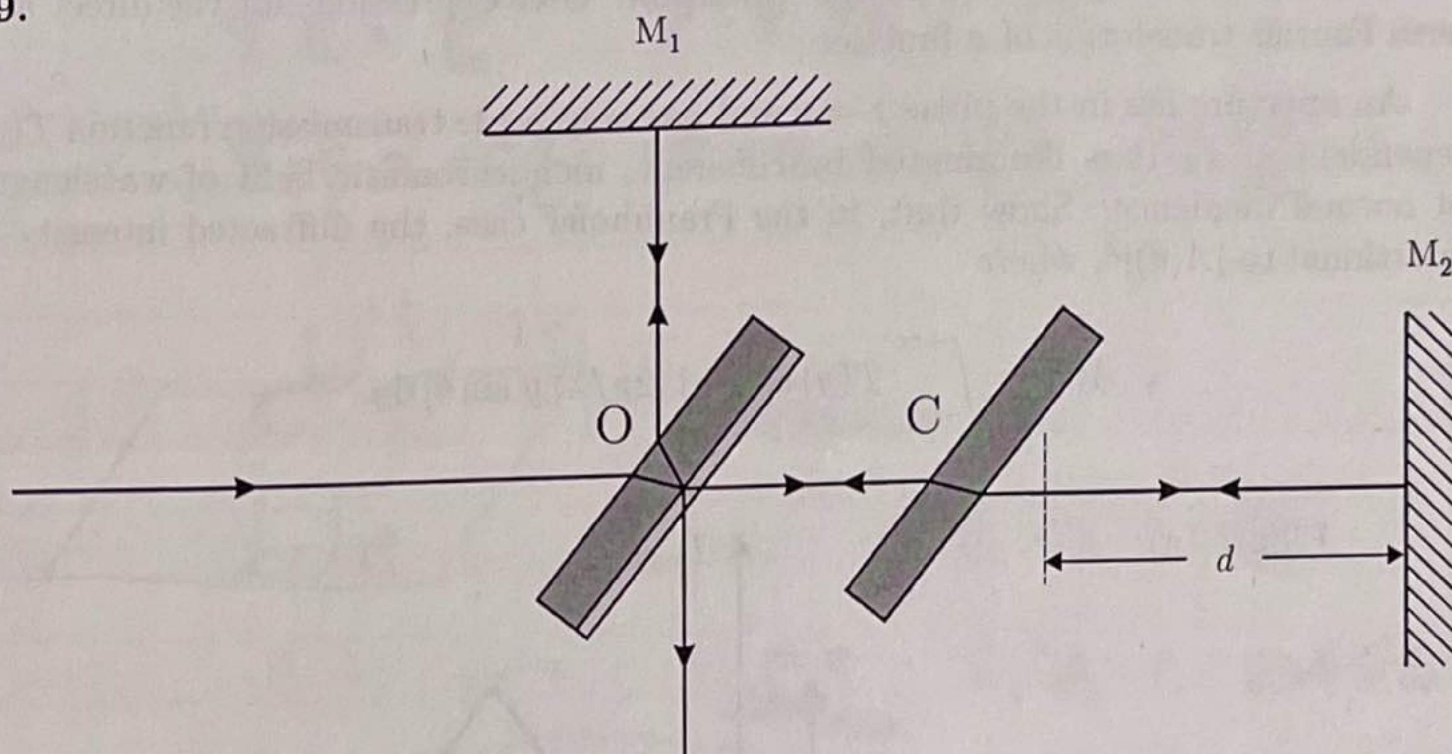
The figure shows the elements of a Michelson interferometer: O, a half-silvered glass plate; C, a glass plate; M<sub>1</sub>, a fixed mirror; and M<sub>2</sub>, an adjustable mirror which can be moved towards or away from O. Also shown are paths of rays in a collimated beam from a coherent, monochromatic light source of wavelength  $\lambda = 500 \text{ nm}$ . Explain the functions of elements O and C. Explain why interference fringes are formed and describe how they might be observed.
