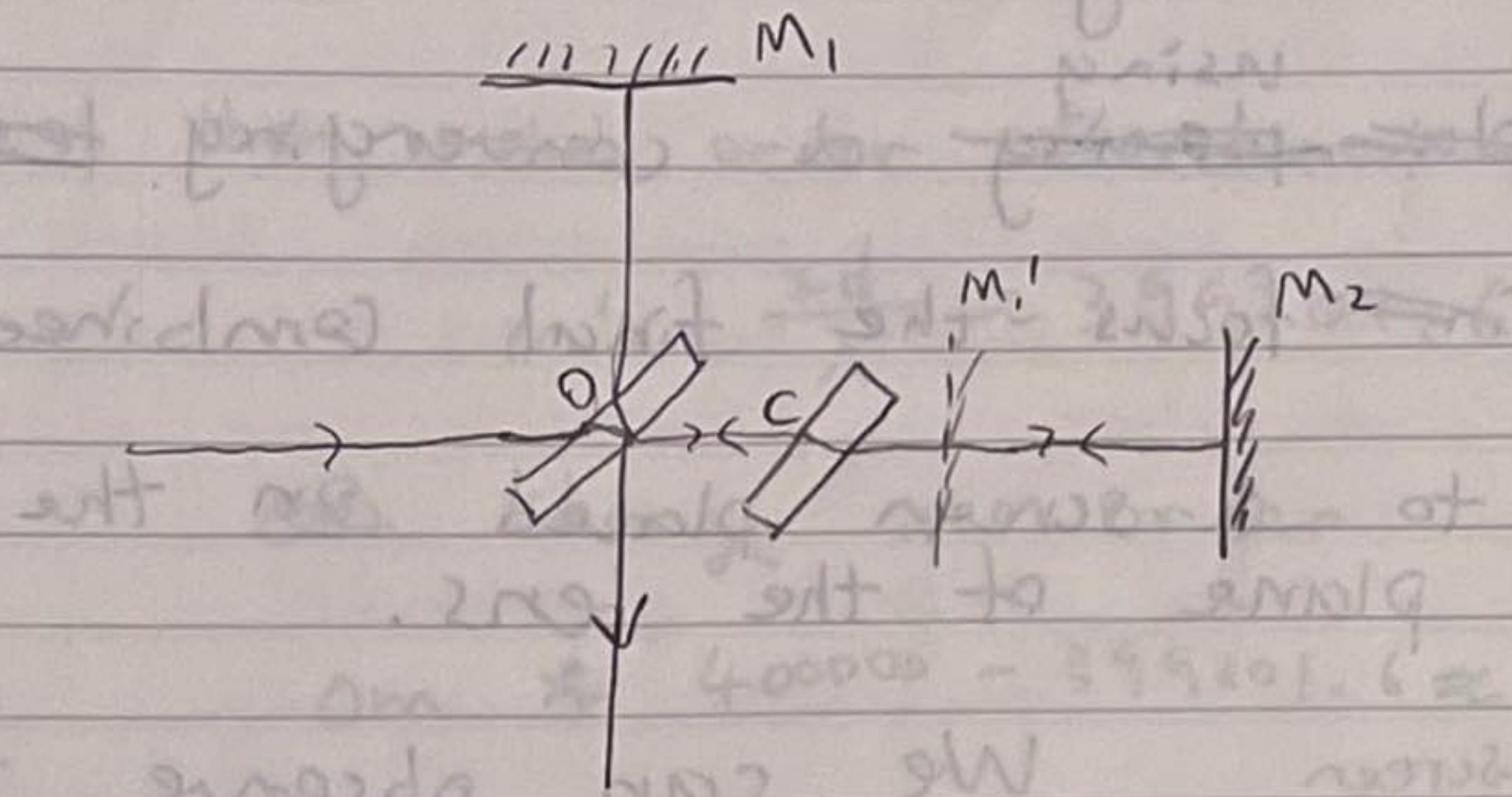
→ O is used as a beam splitter to ~~split~~ split the incoming light beam into two beams that hit  $M_1$  and  $M_2$  respectively. It also introduces a phase shift of  $\pi$  between the two beams as the two sides of the Beam Splitter have different change in refractive index (one from small to large, the other from large to small)
