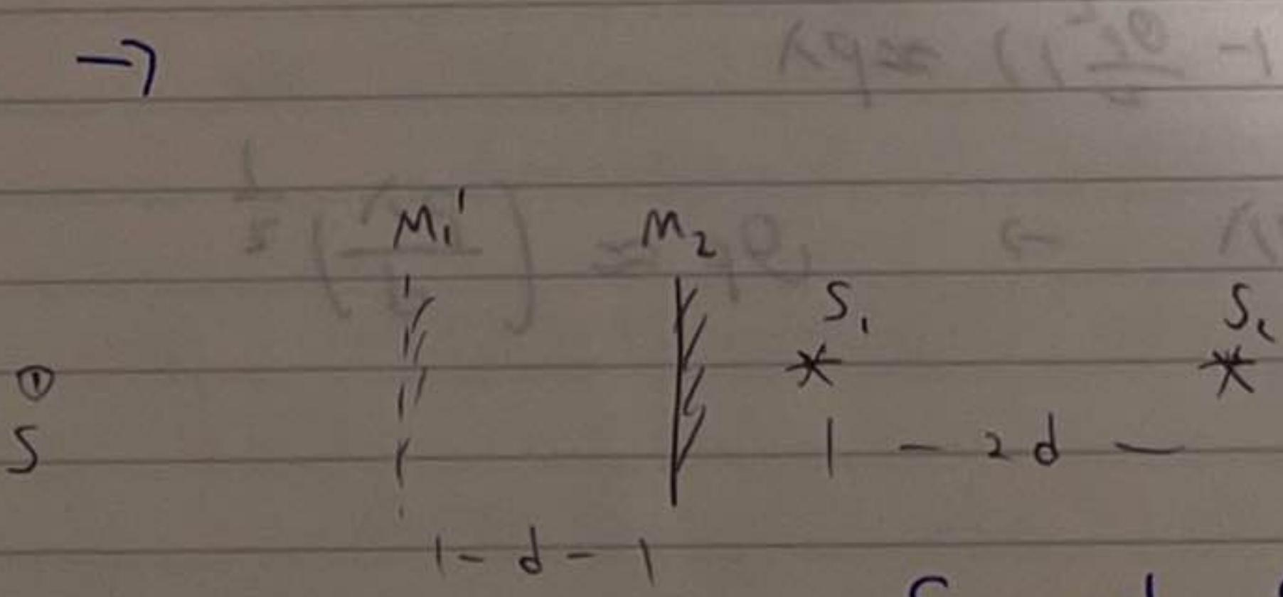
→ The image of mirror  $M_1$ ,  $M_1'$ , and the mirror  $M_2$  together form two images of the light source  $S$ , namely  $S_1$  and  $S_2$ .
