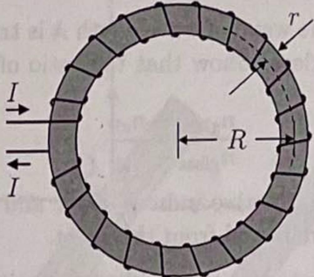
The figure shows a coil of copper wire wrapped around a torus of material. The copper wire makes  $N$  turns and carries a current  $I$ . The torus has a major radius  $R$  and a minor radius  $r$ , where  $r \ll R$ . Assume that the magnetic field is entirely within the material.
