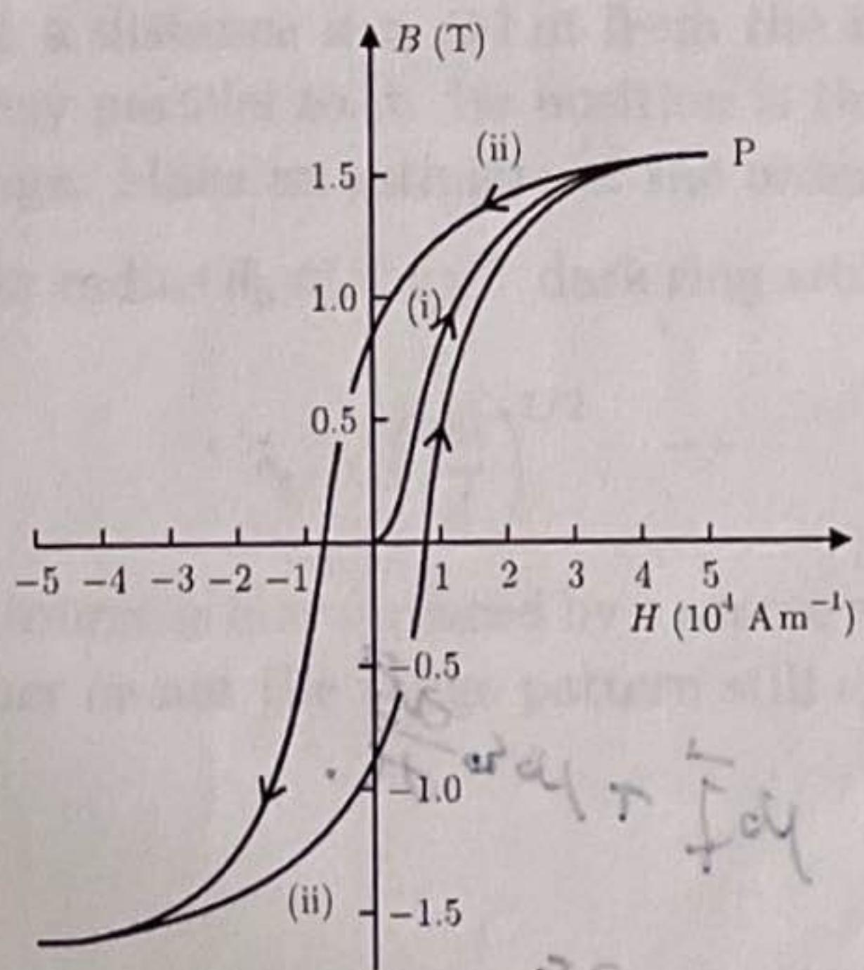
The graph shows the experimentally measured relationship between  $H$  and  $B$  as the material is first magnetized along curve (i) to point P, and then taken around the hysteresis loop (ii). Given that  $R = 0.2$  m and  $r = 0.02$  m estimate the energy needed to magnetize the material and the energy needed to take the material around the hysteresis loop. [7]
